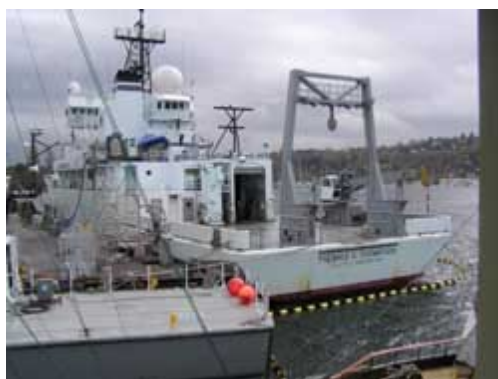
15T telescopic crane, 60 feet long, on oceanographic vessel
