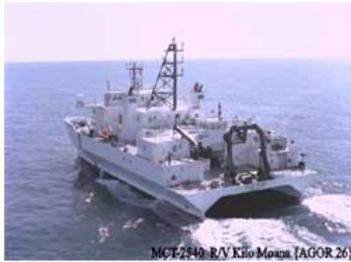
25T telescopic crane, 40 feet long, on AGOR 26 research vessel R/V Kilo Moana
